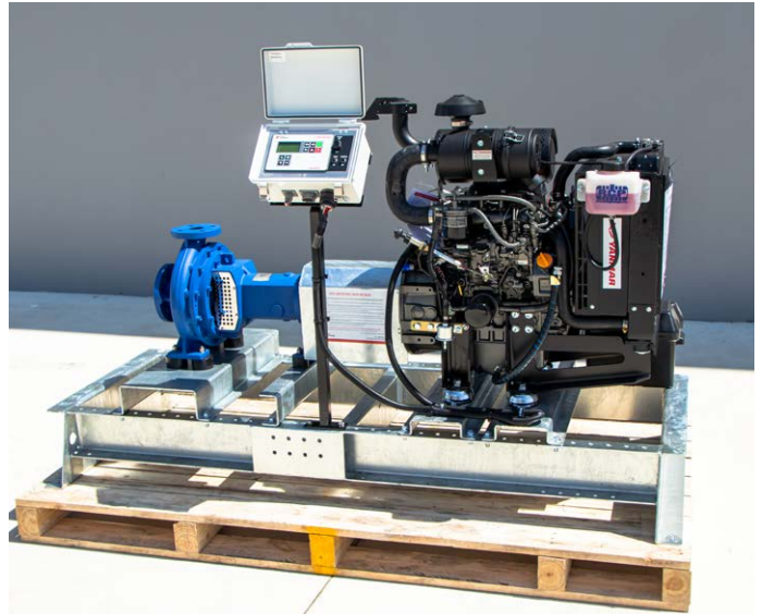
One of Brown Brothers Engineers' recent custom-built pump sets.
